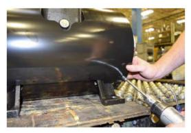
(Fan Cooled Only) Remove the fan shroud supports connecting the shroud "tin" to the rear endplate.
