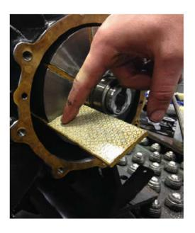
8. Inspect the original vanes for any delamination, chipping or other damage.
