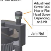
Tighten adjustment screw (CW) until it seats on the cam. (Do not force!
