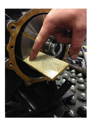
Inspect the original vanes for any delamination, chipping or other damage.
