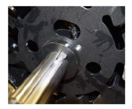
27. (Fan Cooled Only) Reinstall the fan assembly, the key should be pushed all the way to the end of the key slot on the drive end.
