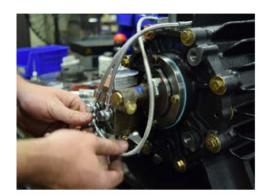
26. Reinstall the oil pump drive key in the non-drive end of the rotor.
