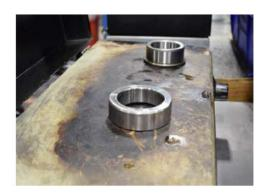
17. (Continuation of Step 15) Remove the two (2) inner races from the replacement bearings provided in your repair kit.
