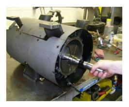
16. Clean the rotor and rotor slots and inspect the rotor for wear or damage.
