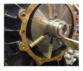
7. Remove the rear endplate with a gentle "wiggle", clean gasket surface and remove the vanes for inspection.
