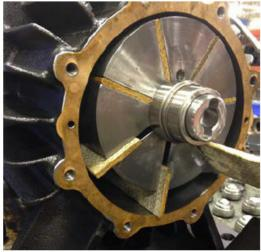
7. Remove the rear endplate, gasket, and vanes.
