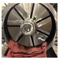
8. Place a cushion beneath the rotor to prevent damage when the front endplate is unbolted (cardboard, rag, etc.).
