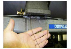
Divert the pull wire into the housing cavity and out through the intake port.
