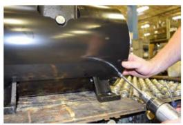
(Fan Cooled Only) Remove the eleven (11) self-tapping screws that fasten the fan shroud "tin" to the pump.
