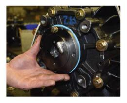
Remove the four (4) bolts that hold the rear bearing cover to the rear endplate and note that the wave spring seal is to be re-used.
