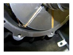
Shift the housing so that the intake (Square port) is hanging slightly off of the rebuild work surface.
