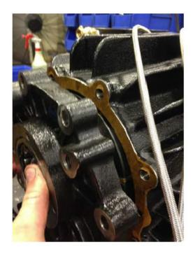
9. Install one (1) new endplate gasket between the housing and the endplate, do not use any gasket sealer.
