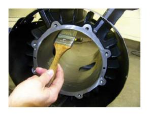
14. Clean the housing of any debris and apply a liberal amount of lubrication to the housing bore.
