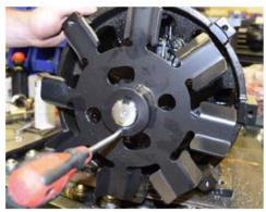
9. (Fan Cooled Only) Remove the fan guard on the drive end side of the pump. Remove the fan and key from the rotor drive end by first loosening the fan hub screw. You may find it necessary to drive the hub apart with a screw driver in order to slide the fan assembly off of the rotor.
