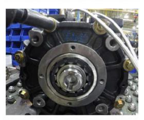
Remove the top two (2) bolts that hold the rear endplate to the pump housing and replace with two (2) 3/8-16 threaded dowels. Once in place, remove the lower six (6) 3/8 hex bolts.
