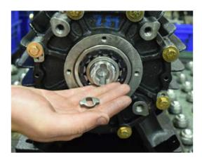
Remove the oil pump drive key from the end of the rotor.
