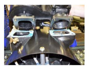
28. Install two (2) four-way gaskets to the housing interface.
