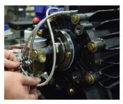
Remove the oil pump guard. Disconnect all oil lines feeding from the oil pump
