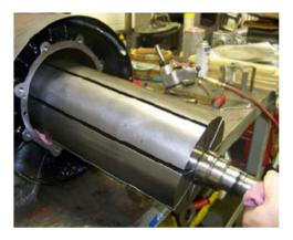
11. Gently guide the front end plate off of the (2) 3/8-16 threaded rod segments to fully settle the rotor body on the base of the housing bore.
