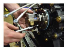
2. Remove the oil pump guard. Disconnect all oil lines feeding from the oil pump
