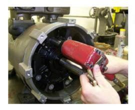
Repeat step 6 to drop the rear end of the rotor down onto the cushion.
