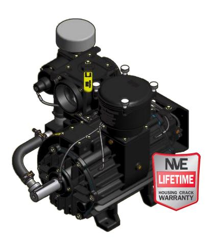
\*The maximum allowable operating vacuum will vary depending on R.P.M., ambient temperature, altitude and time running. The basic principle to keep in mind is - faster R.P.M., higher air temperature and longer run time all equal more heat in pump. When installing an NVE 866 pump we recommend a normal R.P.M. of 1000. Other speeds are OK as long as exhaust gas temperatures read on the supplied thermometer do not exceed 380 degrees F.
